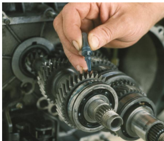
Figure 2. Restoration of rolling bearing fit
