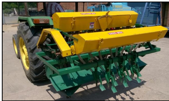
Figure 5. Developed raised bed inclined plate onion planter
