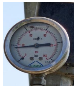
Slika 4. Radni pritisak na ulazu u mašinu Figure 4. Working pressure at the machine inlet
