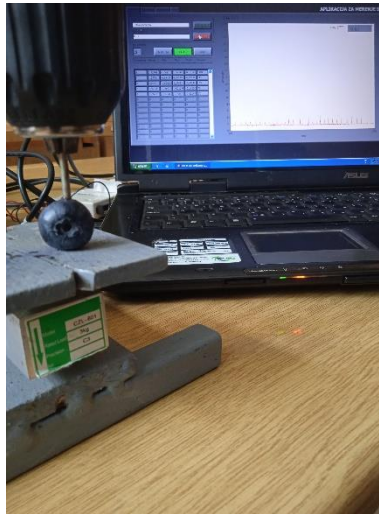
Slika 1. Uređaj za merenje čvrstoće ploda metodom probijanja Figure 1. Device for measuring fruit firmness using the method of puncture
