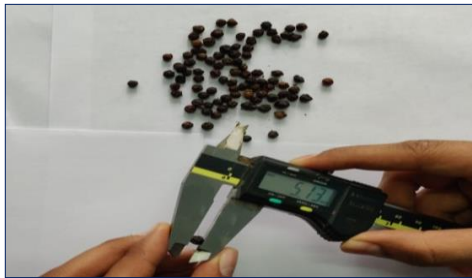
Fig.1. Measurement of size of black pepper seeds by digital Vernier Caliper
